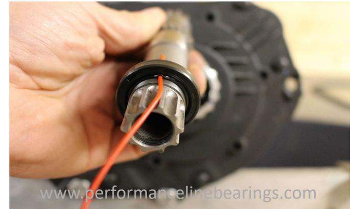
Step 7, Ensure the tool you use fits over the crankshaft all the way down to the bearing. Pass the wire through the tool and push the seal until it stops at the bearing.
