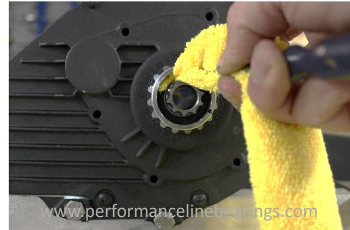
Step 3, Apply a thin film of silicone or water resistant grease
