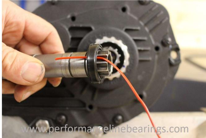
Step 6, The wire is to let the air escape as the seal is pushed in. If you don't have the crankshaft fitted, this step is not necessary.
