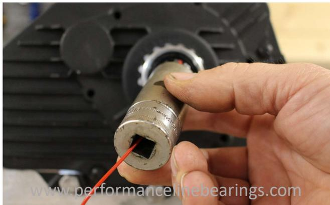
Step 8, With the seal in place past the circlip groove, the wire can be pulled free. Push the seal once more to ensure it is fully seated.
