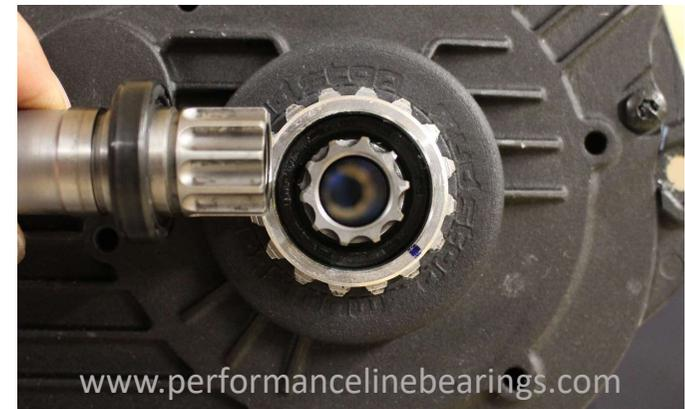
Step 9, Re-fit the crankshaft outer circlip.
