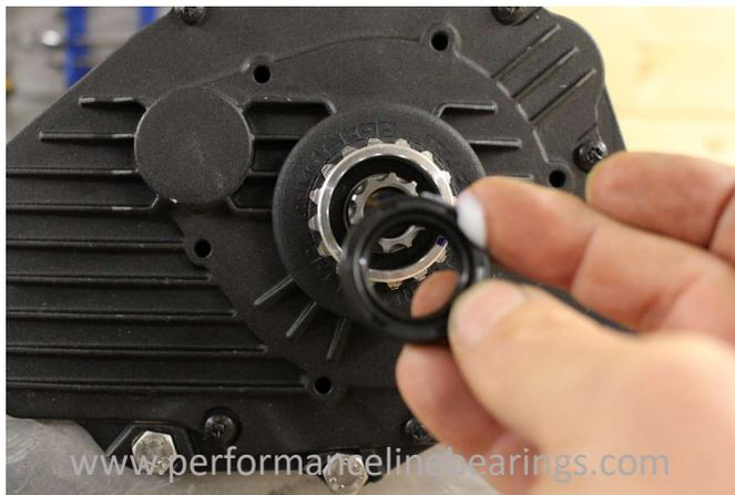
Step 4, In with your seal is 100mm length of 1mm thick Wire. Place this wire through the seal and along the crank
